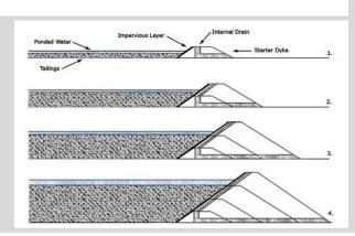
The tailings facility of the Volta Grande mine in Brazil is designed using a Downstream design and is engineered using compacted earth and rock fill. Our tailings design is <u>not</u> constructed with tailings.
