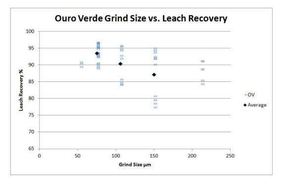
Figure 13-12: Grota Seca Gold Leach Recovery vs Grind Size
