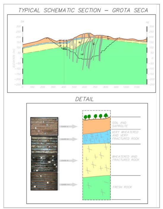
Figure 16-2: Typical Geomechanical Section – Grota Seca
