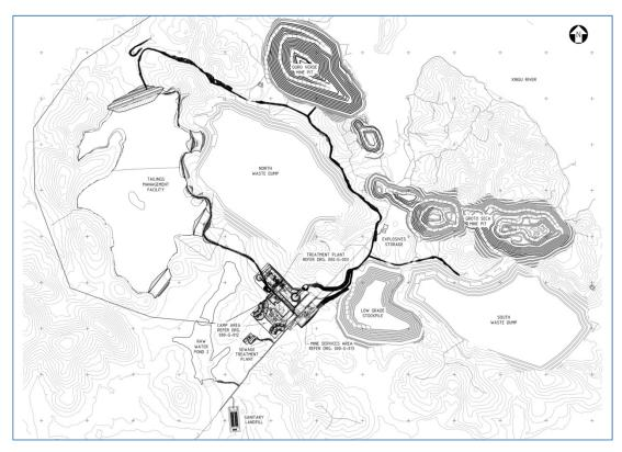
Figure 1-1: Site Layout with Open Pits and Waste Management Facilities
