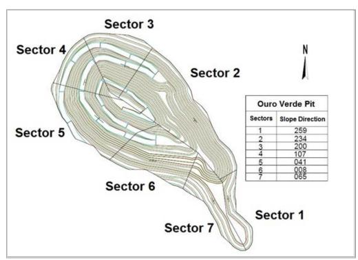
Figure 16-3: Pit Slope Sectors – Ouro Verde Pit
