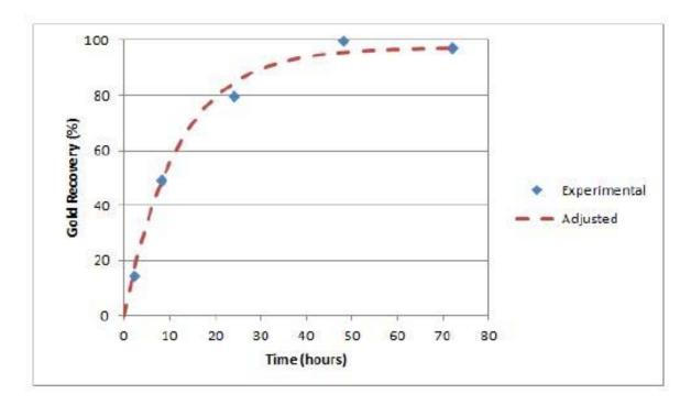
Figure 13-7: Saprolite Leaching Kinetics at P<sub>80</sub> 75 µm and 550 pm CN<sup>-</sup>
