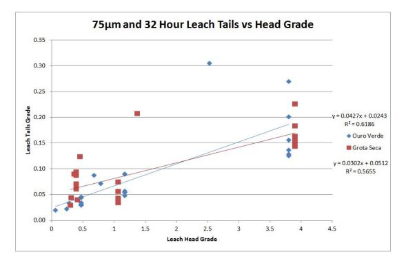
Figure 13-18: Gold Recovery Curves at Design Conditions of 32 Hours and P<sub>80</sub> 75 um
